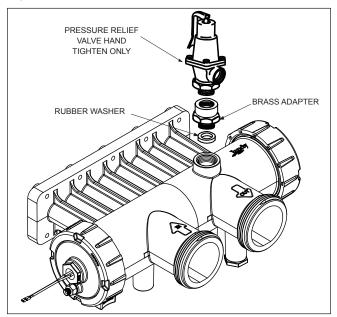
Figure 14. Pressure Relief Valve Installation
