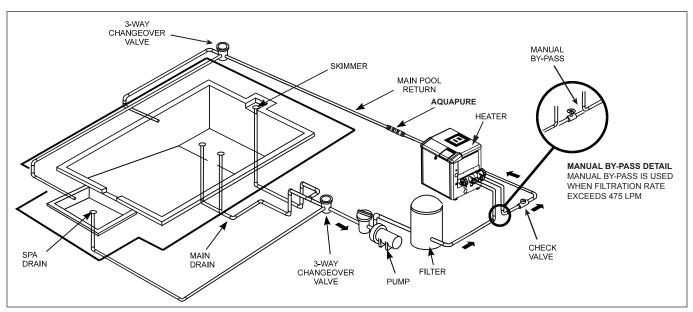
Figure 6. Typical Piping Installation
