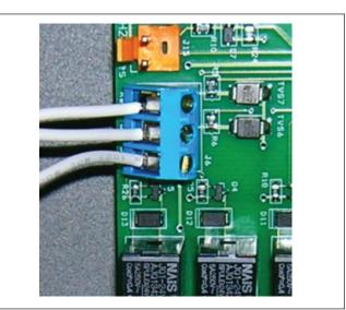
Figure 16. Remote Pool-Off-Spa Connection (3-Wire Connection)
