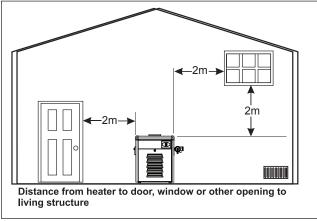
Figure 3. Outdoor Heater Installation
