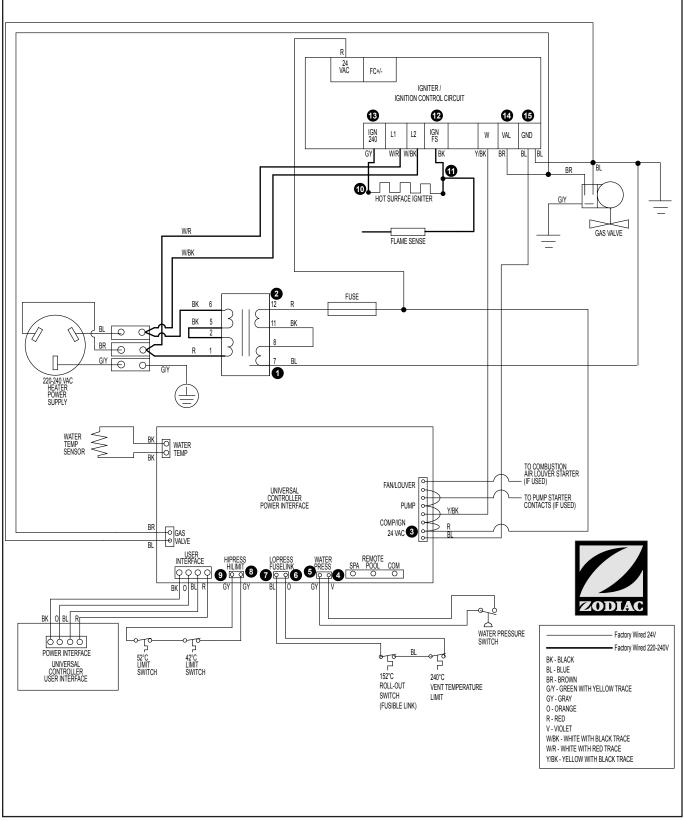
Figure 26. Test Point Identification Diagram
