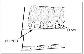
Figure 22. Main Burner Flame
