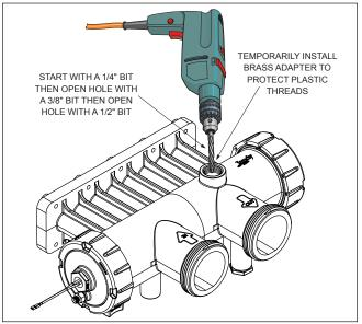
Figure 13. Drill Hole for Pressure Relief Valve
