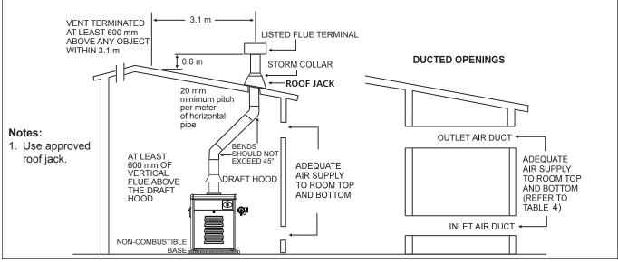
Figure 4. Indoor Installation Venting or Outdoor Shelter Venting
