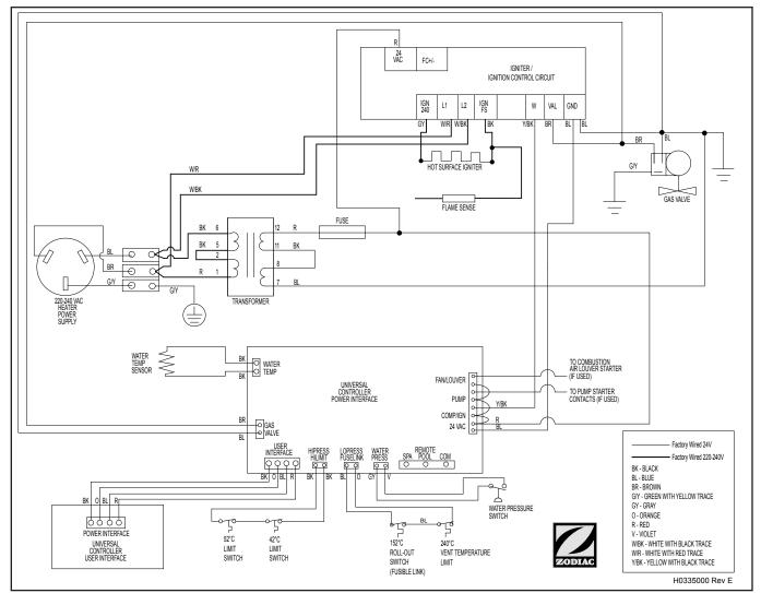
Figure 15. Legacy Model WLRZ Electronic Connections/Schematic Wiring Diagram
