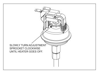
Figure 24. Adjustment of Pressure Switch
