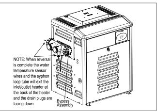
Figure 9. Water Connections Reversed
