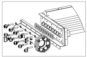
Figure 11. Header Bolt Tightening Sequence
