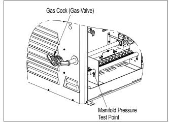
Figure 5. Fitting a Gas cock (gas-valve)
