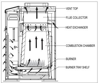
Figure 23. Atmospheric Combustion System
