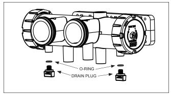
Figure 20. Draining the Heater
