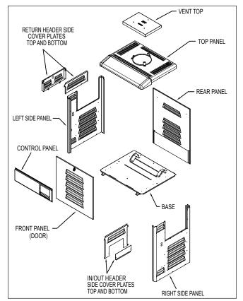
Figure 10. Legacy Model WLRZ Panel Identification
