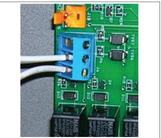
Figure 17. AquaLink RS or Remote TSTAT Connection (2-Wire Connection)
