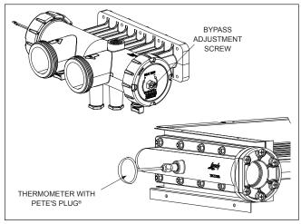
Figure 25. Temperature Rise Measurement
