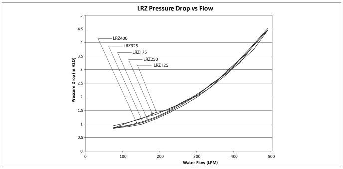
Figure 7. Hydraulic Head Loss Curve
