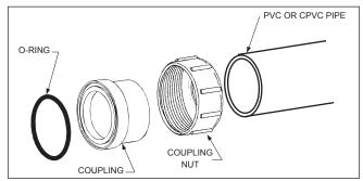
Figure 12. Piping to Heater
