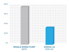
\* 1400 RPM = 70 (LPM) = 0.160 kW/h - 24 hours per day x \$0.25kwh x 365 days x 0.160kw/h= \$350.40
