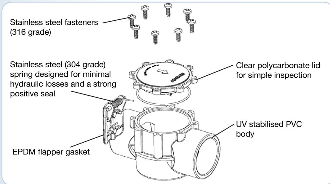
The Flow Check valve's pressure rating of 400 kPa (58 psi) and its 316 stainless steel fasteners make it suitable for domestic and commercial applications.
