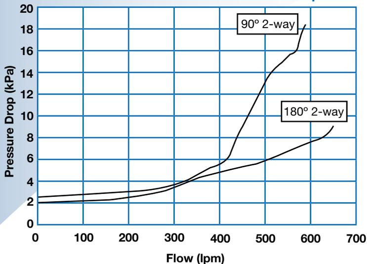
40/50mm Flow Check Valve Pressure Drop
