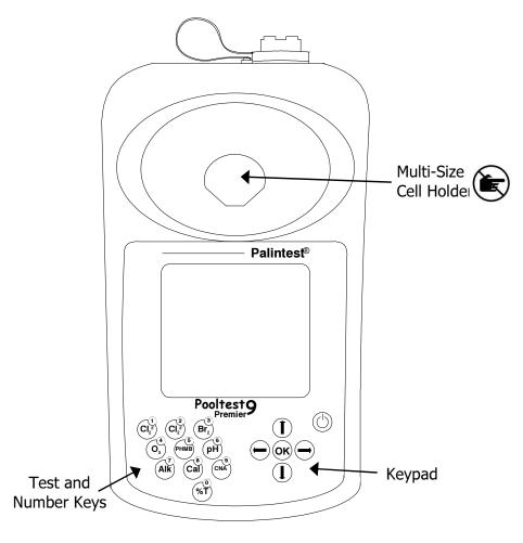
The Palintest Pooltest 9 Premier is a precision photometer specifically developed for testing swimming pool water.
