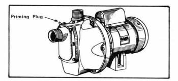
If air has stopped bubbling out of the pump discharge, then the self priming action has ceased. Installation should be checked, pump refilled with water and priming attempted again.
