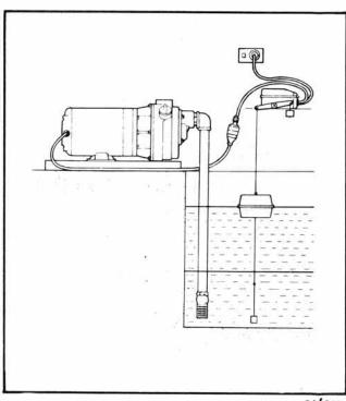
Type of water: Pumps are capable of pumping spetic tank effluent, sink wastes, some dirt or sand, drainage or polluted water and industrial wastes. They are not designed to pump large quantities of foreign matter. If fluid contains large or stringy material, then an adequate suction filter should be used.
