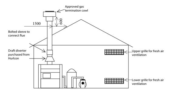
An indoor draught diverter must be purchased from Hurlcon and fitted to unit in accordance with AstralPool's instructions and Installation Codes before the heater can be enclosed.
