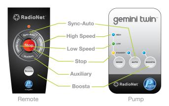
**AUTO mode:** Automatically changes speed between HIGH and LOW on each power-up to enhance effectiveness of pool cleaning equipment.
