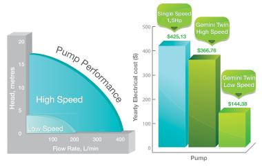
\*Annual pump operating cost is based on turning over an average size pool of 50,000L twice per day at \$.20 per kWh.
