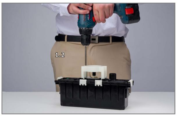
Step 1.2 Secure the impeller protector cylinder with 4 KA50X12 screws.
