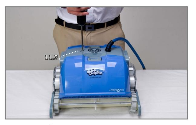
Step 11.3 Secure the impeller cover with a KA50X12 screw.
