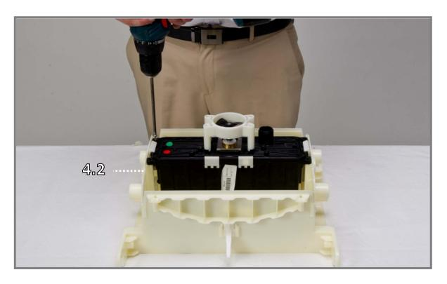
Step 4.2 Secure the motor unit to the frame with 4X KA50X20 screws.
