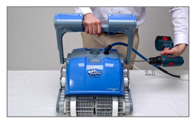
Step 1.1 Unscrew the 2 screws holding the handle in place.
