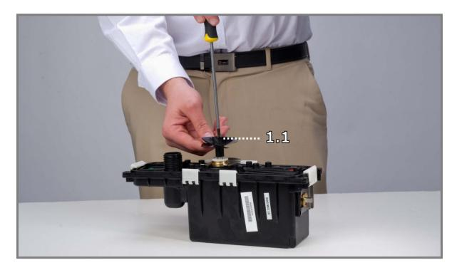
**Step 1.1**Secure the impeller with a 4X25 screw.
