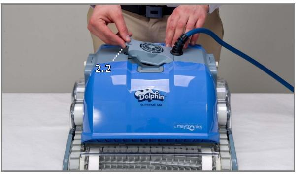
**Step 2.2**Lift the impeller cover up from one side and then take it off.
