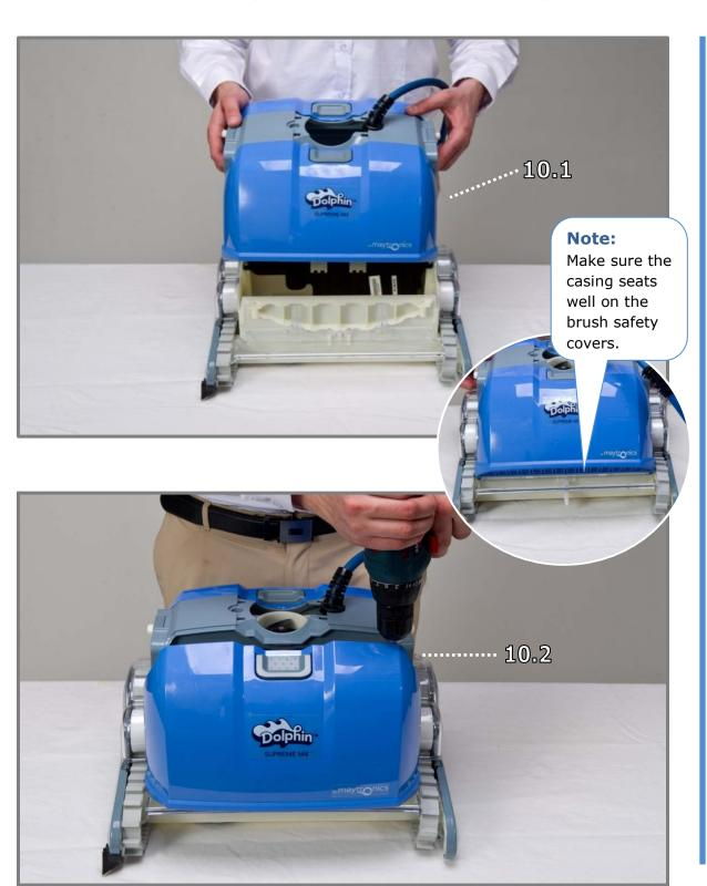
**Step 10.1** Place the outer casing on the frame.
