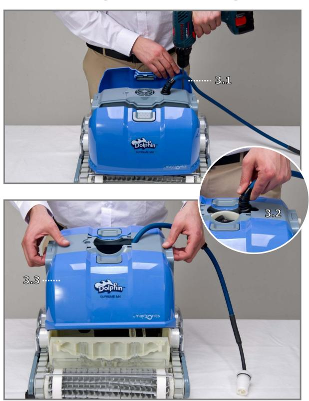
**Step 3.1**Unscrew the 4 screws holding the outer casing in place.
