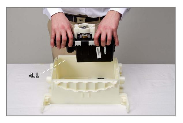
**Step 4.1** There is only one way to place the motor unit in the frame.
