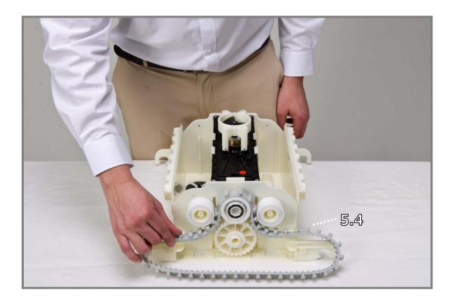
**Step 5.4**Place the track in its place as shown on both sides of the robot.
