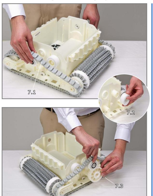
**Step 7.1**Remove the pulley together with the track from one side of the robot.
