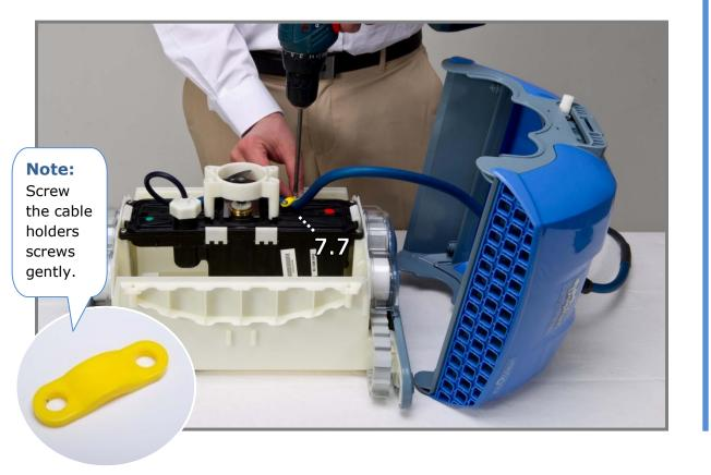
**Step 7.7**Secure the cable holders with 4X KA50X12 screws.
