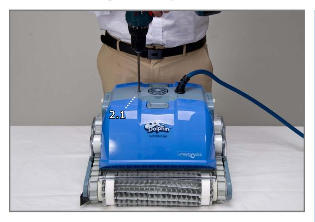
**Step 2.1**Unscrew the screw holding the impeller cover in place.
