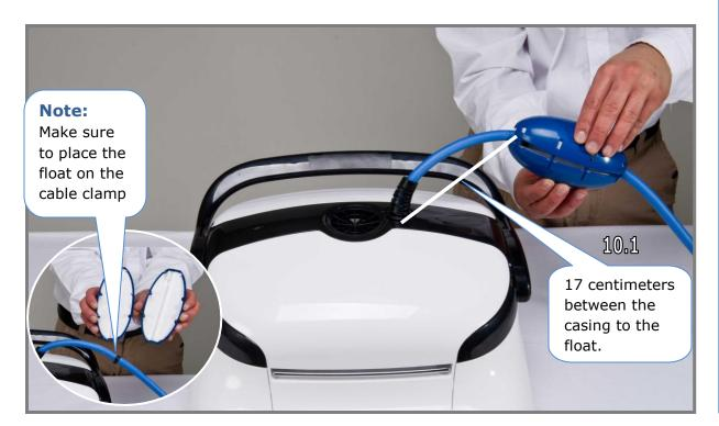
**Step 10.1**Position the cable float 17 centimeters from the casing.
