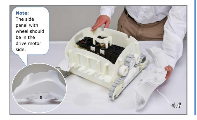
**Step 4.6**Put the side panel with wheel into place.
