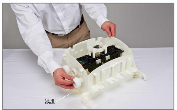
**Step 3.1** Place 2 guide wheels on the opposite side of the drive motor shaft.
