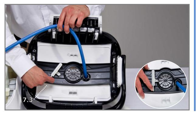
**Step 7.3**Secure the impeller using the impeller locker.
