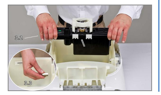
**Step 3.2**Remove the motor unit.
