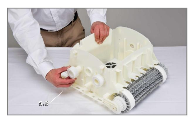
**Step 5.3**Remove the guide wheels from both sides of the robot.
