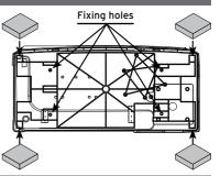
It is possible to fix the appliance to the ground using the holes in the base of the appliance or using fixing rails (not supplied). It is also possible to fix the appliance with brackets (not supplied).
