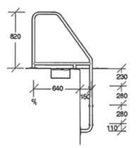
Rod re-inforced moulded ladder treads 500mm wide Extra wide for level deck with gutter For sloping wet deck with gutter price on application and drawing is required.
