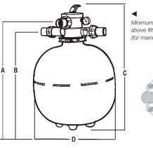
Minimum height clearance above filter 600mm (for maintenance purposes)
