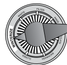
Fig. 11: Valve setting for winterstorage. Stop pump beforechanging valve position.
