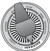
Figure 9: Valve settings for startup. Stop pump before changing valve position.
