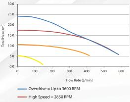
Medium Speed = 2000 RPM Low Speed = 1125 RPM
