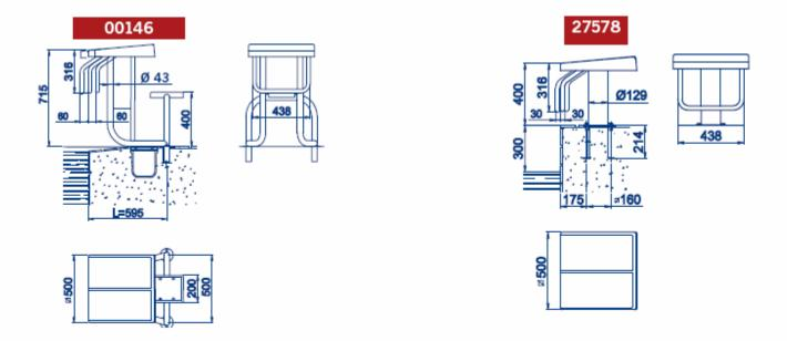
Note: The 00146 platform can be manufactured, made to order, for adapting it to overflow level. In the case the distance L must be given.
