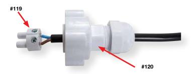
**Step 4.** Slide #119 Female Plug into #120 Connector Housing, be sure to align the keyway on #119 Female Plug with keyway on the inside of the #120 Connector Housing.
