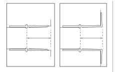
Do not install in fittings with less than 0.89" (22.6mm) of depth. IF the distance is between 0.89" and 1.26" — Mod-Lite will fit. IF measured between 0.89" and 0.94" — Remove the foam spacer IF measured between 0.95" and 1.26" — Keep the foam spacer
